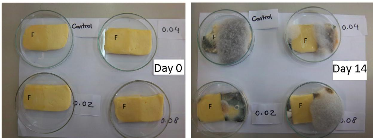
**Fig. 2.** Samples of soft cheese partially coated with triticale flour films (control and with different concentration of natamycin) at 0 and 14 days of storage at room temperature. F: film; 0.02: film containing 0.02% natamycin; 0.04: film containing 0.04% natamycin; 0.08: film containing 0.08% natamycin.
