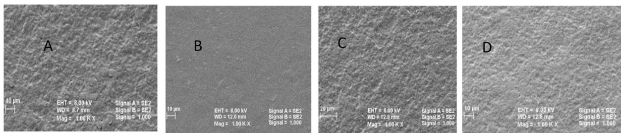
**Fig. 1.** Scanning electron micrograph (SEM) of surface of triticale flour films. A: Control film. B: film containing 0.02% natamycin. C: film containing 0.04% natamycin. D: film containing 0.08% natamycin.
